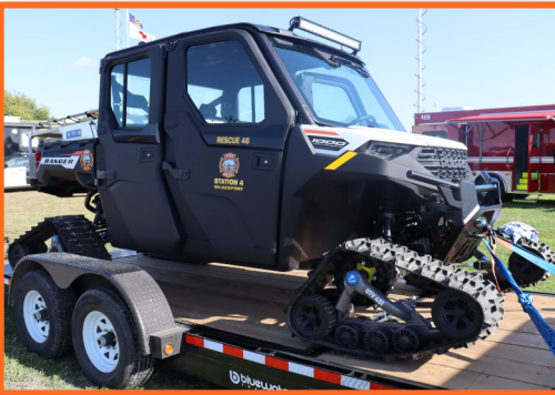
Above: Modern tractor-like vehicles such as this utility task vehicle (UTV), a 2023 Polaris Ranger that responds from Station 4 Wilkesport, is used to answer the numerous emergency calls in areas not accessible by fire trucks. It carries a pump-equipped water tank for fire suppression operations and a compartment for carrying a backboard for rescue operations.
